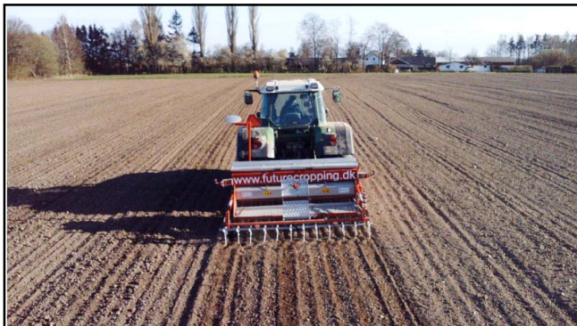
Fig. 2: GNSS-assisted coulter depth control system for a low-cost seed drill.
